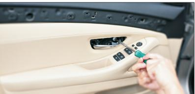
3. Note that the door panel is fixed by numerous plastic clips, carefully pry away the door upward and disconnect all wiring and door latch cables. Be very careful to avoid the damage of the plastic clips during the door panel dis-assembly.
