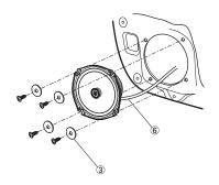
• Install the speaker into the vehicle by using vehicle pre-fitted screw and included speaker cable ⑥.
