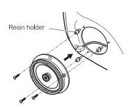
• Resin holder should be removed after taking the speaker out.
