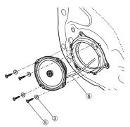
• Install the speaker by using included speaker cable ⑥.
