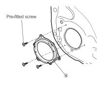
• Install the adaptor 4 into the vehicle by using pre-fitted screw.
