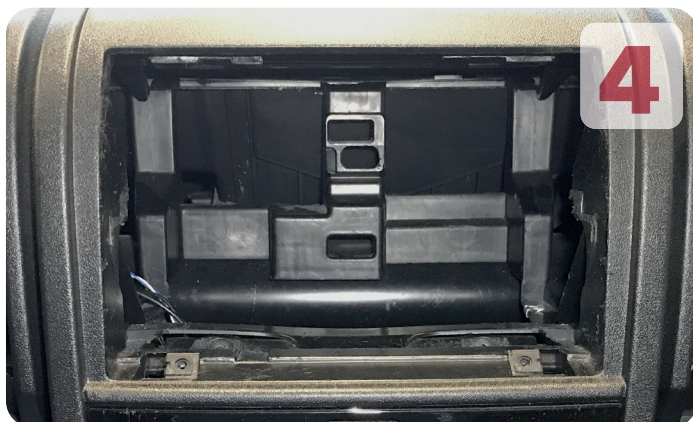
Dashboard after cutting
