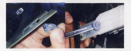
FASTEN THE PLASTIC HOLDER ON THE METAL PLATE SUPPLIED USING THE OEM SCREW AND CLIP
