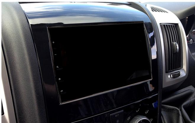
Once the kit has been assembled and the wiring for the stereo is completed, simply use the clips within the kit on the reverse of the fascia and proceed to clip it into place.
