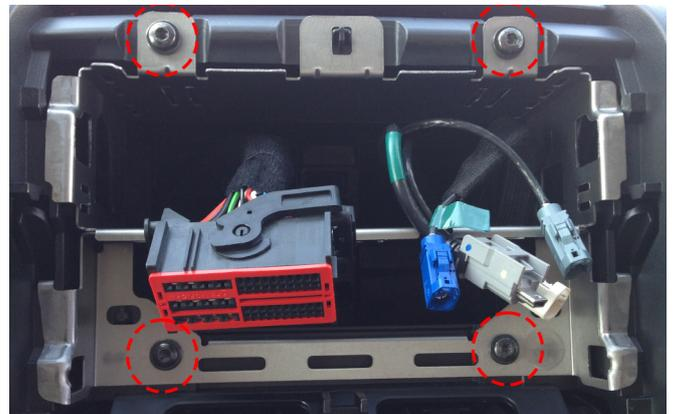
Once the main head unit is out of the way, proceed to remove the highlighted screws. When done, proceed to fully remove the cage.
