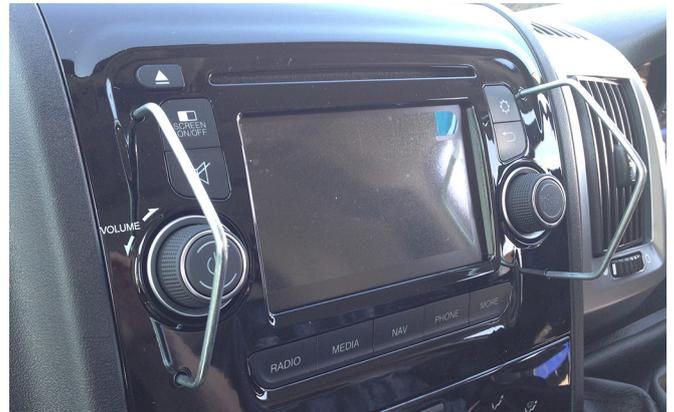
Use a set of release keys to pry the head unit out of the dashboard. Dependent on the style of unit you have installed, you will need either single or double DIN keys. Once released, take out the unit and disconnect all the wiring.
