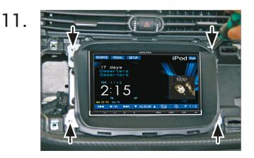
With kit assembly performed correctly, make all of the connections to the stereo and install into the dashboard. Once seated correctly, secure the unit by using the pre-existing screws.
