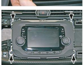
With all of the screws removed, use a panel removal tool to disengage the main fascia panel and remove it whilst disconnecting the side button connector(s).
