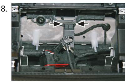
The highlighted area(s) will need to be cut out of the dashboard in order to allow the new double DIN unit to sit correctly.
