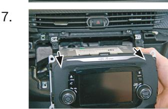
With the screws removed, begin to pull the radio out of the dashboard and disconnect all of the wiring.
