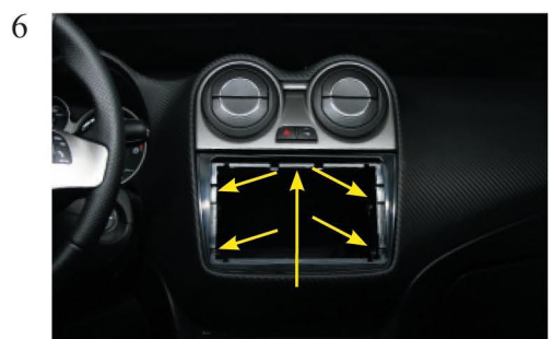
Place the fixing trim and tighten this by five Torx T25 screws.
