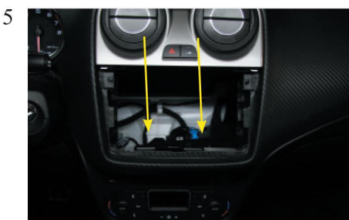
Replace the black box. Make sure you have enough room to place the 2-din headunit.
