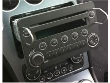
Remove the original radio using the radio release keys.
