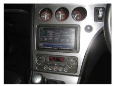
Fit the head unit into the cage, then fit the replacement panel.
