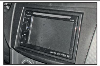
Once all of the wiring has been completed, take the fascia/head unit combination and install it into the dashboard, reassembling the vehicle in reverse order to complete the installation.
