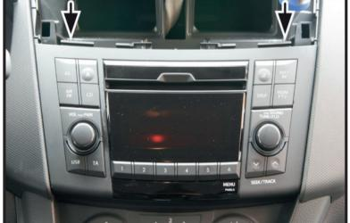
Once free, pull the head unit forward and disconnect all of the wiring.
