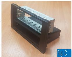
Push the single DIN stereo into the cage until it clips into place
